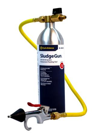
The Flushing Tool contains a reusable canister (with built-in 200psi pressure relief valve), system hose and flush nozzle Gun. Use Flushing Tool to clean line sets for conversion from R-22 to R-410A (mineral oil to POE oil) as well as to flush the contaminants from a system after a compressor burn out. With high acidic levels after a compressor burnout, more solvent may be required to flush the system.
