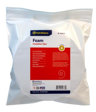
Foam Insulation Tape is a high density cross-linked polyethylene foam coated with a high performance rubber based adhesive. This adhesive system exhibits consistent quick-stick sealing that outperforms the competition. It will effectively insulate either hot or cold surfaces and may be used in a wide range of applications. It is effective at temperatures of -20°F (-29°C) to 160°F (71°C).
